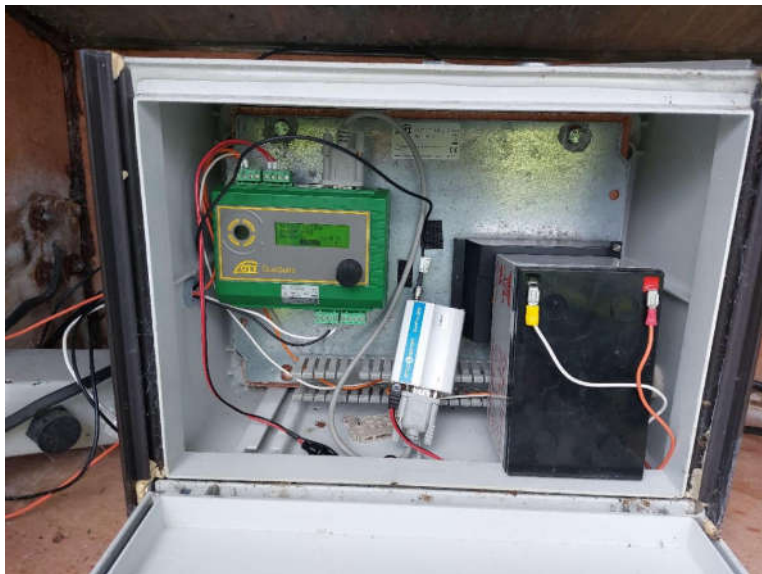
Plate 3 Aggard Bridge 29010 Data Logger
